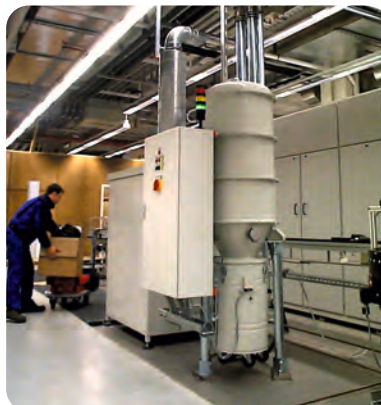
Cyclonic filter FZ-1003 with 100 Litre collection container
